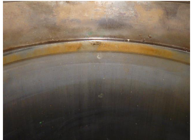
Poor Conditions specially no uniform touching with Liner and piston ring. 内面当たり不良
