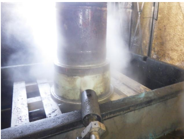
High pressure cleaning. 高压洗淨
