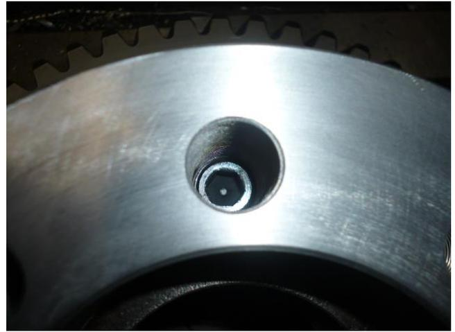
ネジロック塗布 ネジ込み Reverse gear defective joint Distance fixing at 6 bolts.
