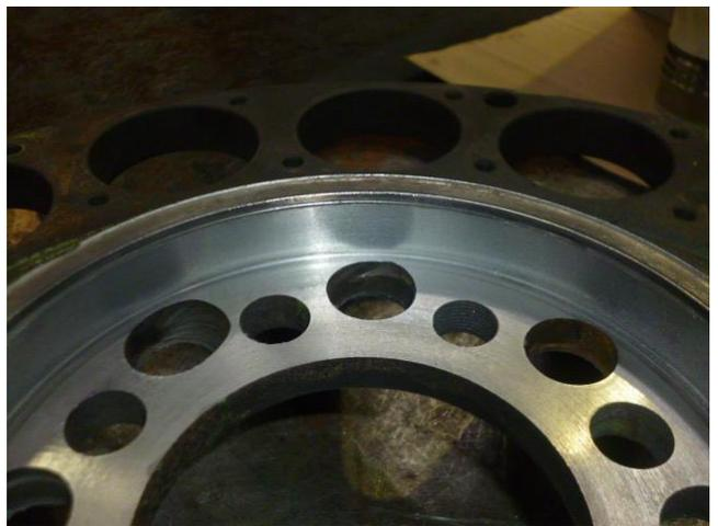
Thickness 35t Depth 20mm Machined up.
