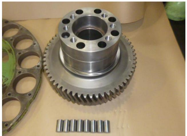
加工完成、洗浄 Processing completed Fixed as Flexible shaft coupling and Reverse gear defective joint 後進歯車
