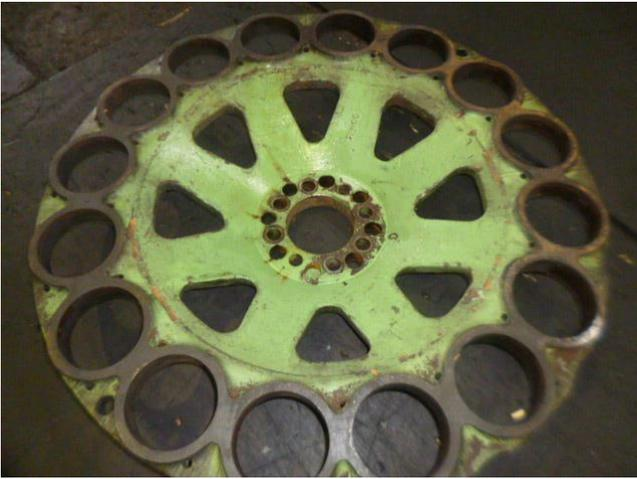
タワミ継手表側。Flexible shaft coupling front side.
