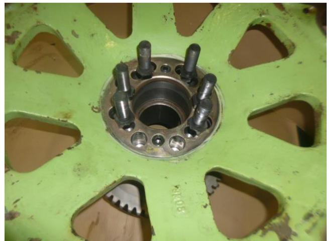
Assembly confirmation Flexible shaft coupling and Reverse gear defective joint
