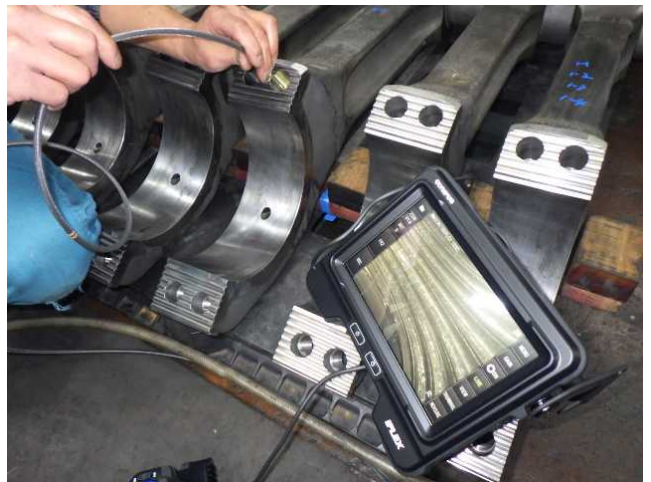
本体側メネジ 内視鏡にて確認 Connecting rod screw part crack magnaflux inspection.
