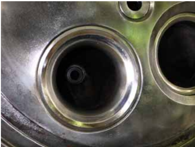
Exhaust valve seat fitting face wear down. 排気弁座 当たり面摩耗
