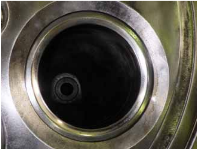
Intake valve seat fitting face wear down. 吸気弁座 当たり面摩耗
