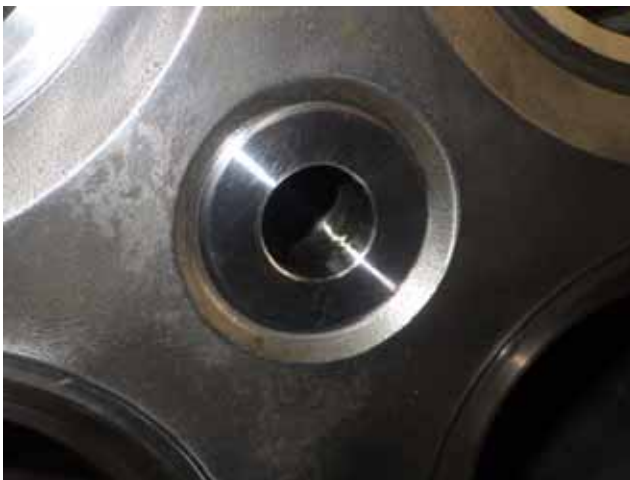
Nozzle sleeve no water leak.
