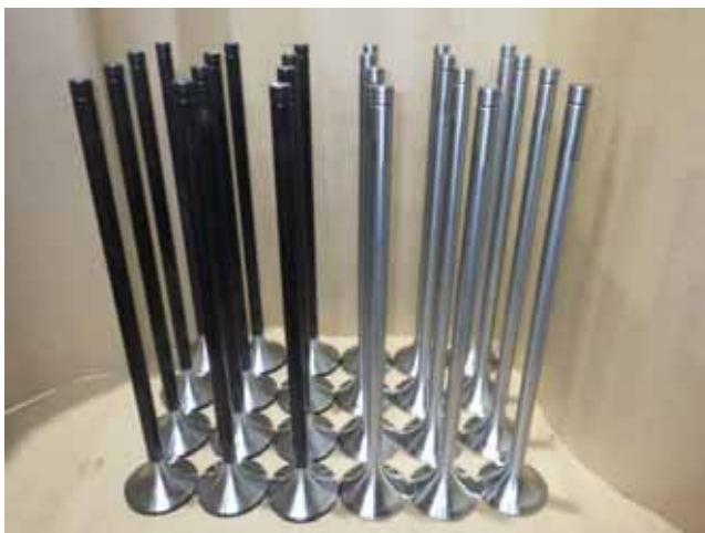
New intake and exhaust valve. 吸排気弁棒新品
