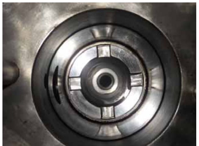
Renewed exhaust valve seat. 排気弁座新替
