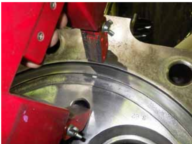
Magnaflux inspection, combustion side.
