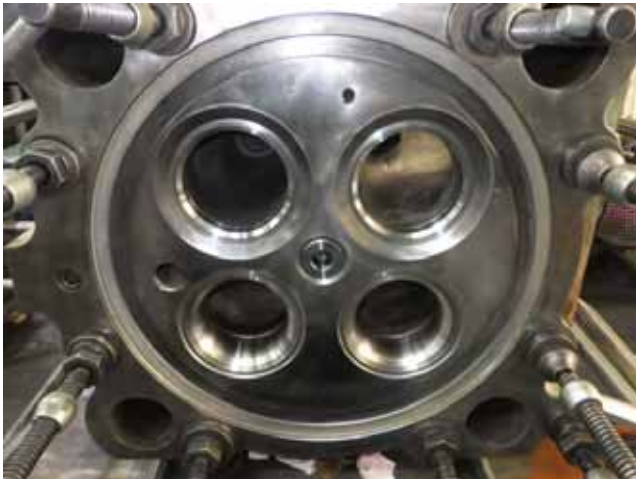
Combustion side no water leak.
