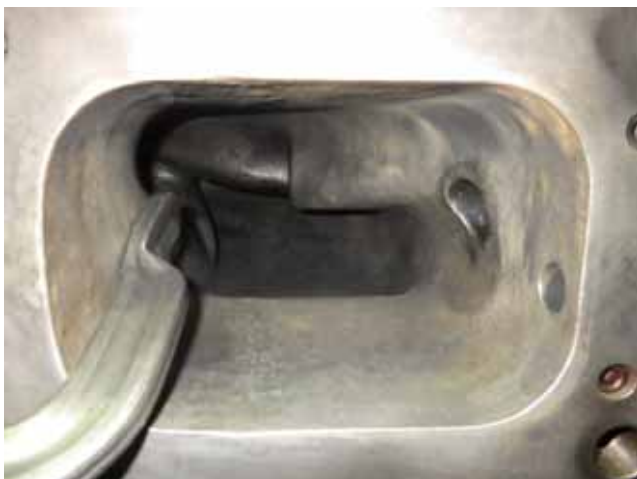
Exhaust port no water leak.
