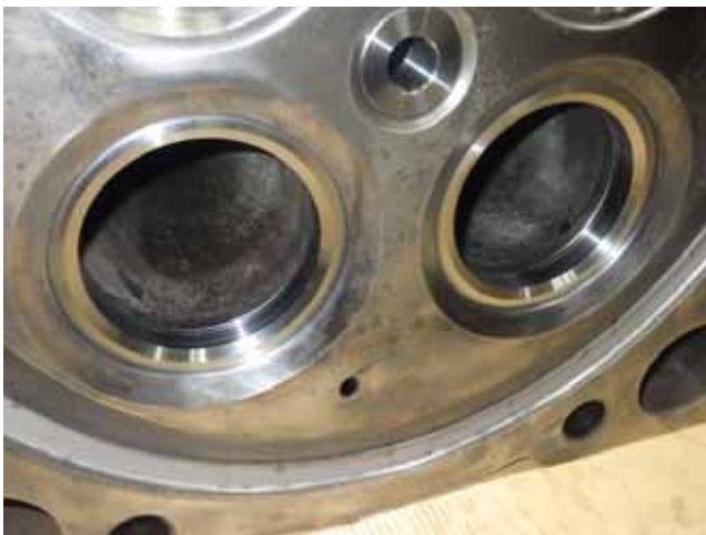
Renewed intake valve seat. 吸気弁座新替
