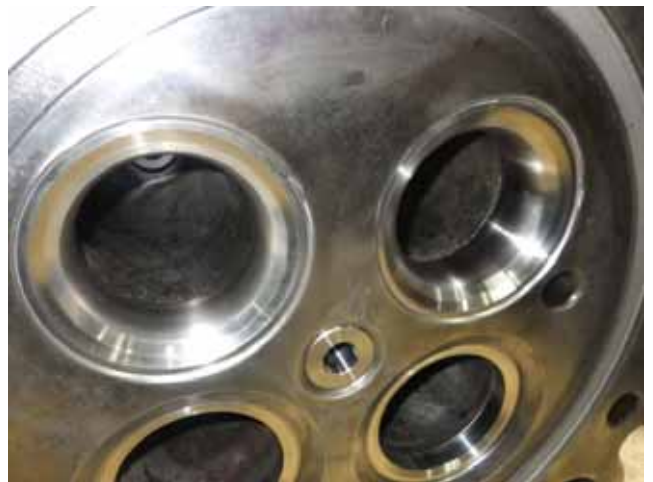
Renewed exhaust valve seat. 排気弁座新替
