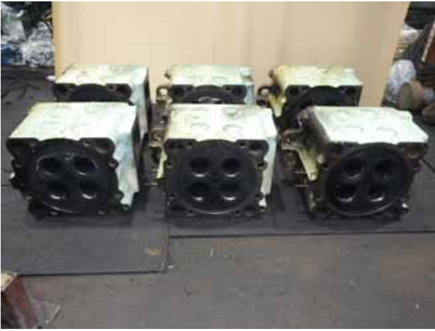
Removed intake and exhaust valve. 吸排気弁抜き取り
