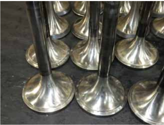
Intake valve fitting face wear down. 吸気弁棒 当たり面摩耗
