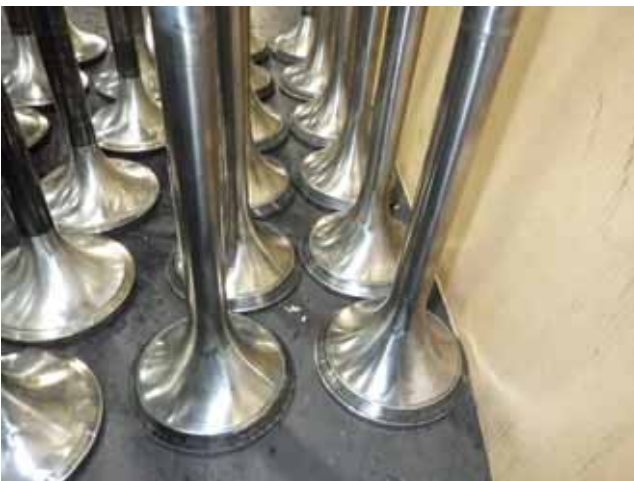
Exhaust valve fitting face wear down. 排気弁棒 当たり面摩耗
