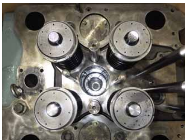
Renewed valve cotter.
