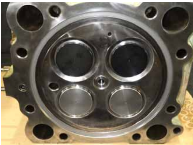
Intake and exhaust valve insertion. 吸排気弁棒組み込み
