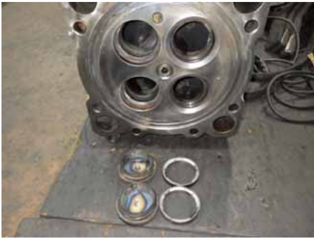
Removed intake and exhaust valve seat. 吸排気弁座抜き取り
