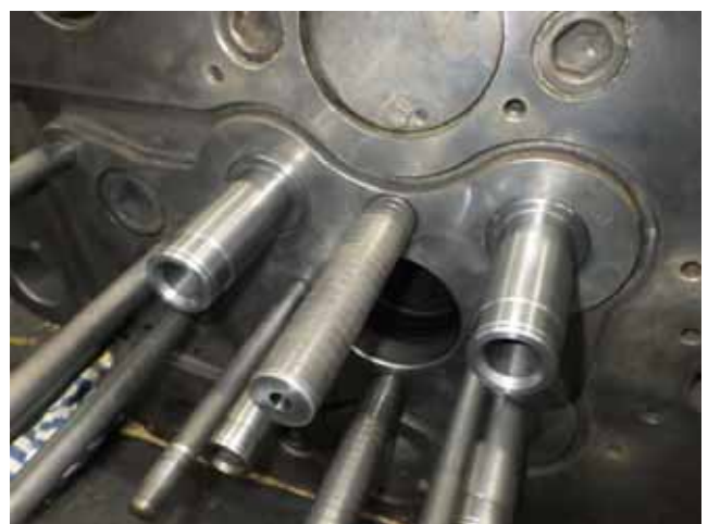
Renewed exhaust valve guide. 排気弁ガイド新替
