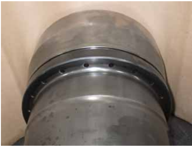
After cleaning cooling water hole. 冷却水孔 洗淨後
