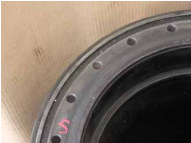
Before cleaning cooling water hole. 冷却水孔 洗淨前
