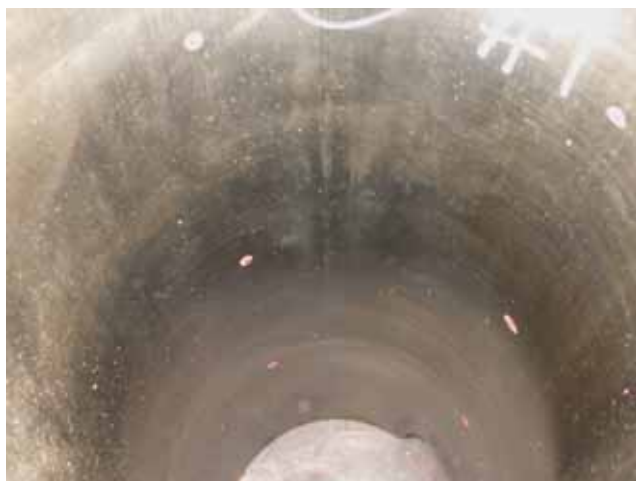
NO.ⓄM210 Poor Conditions specially no uniform touching with Liner and piston ring. 内面当たり不良
