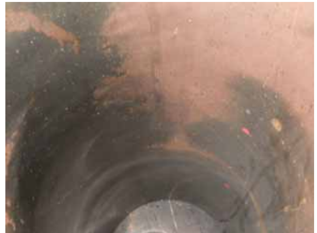
NO.ⓄM216 Poor Conditions specially no uniform touching with Liner and piston ring. 内面当たり不良
