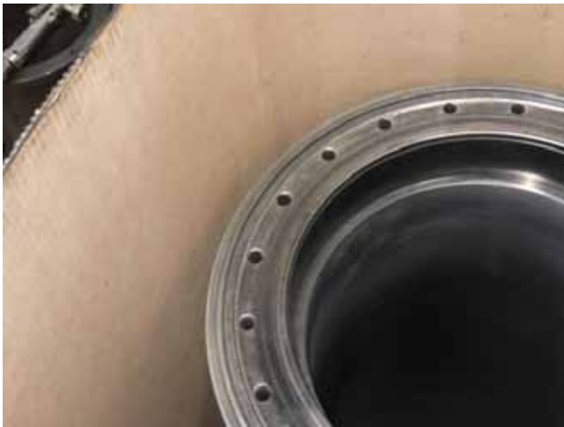
After cleaning cooling water hole. 冷却水孔 洗淨後
