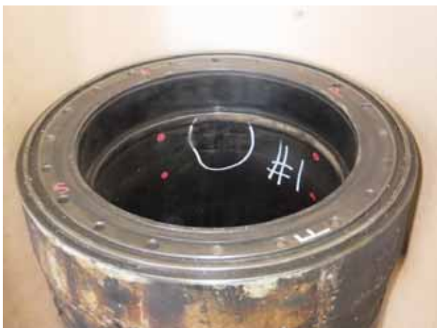
NO.ⓄM210 Poor Conditions specially no uniform touching with Liner and piston ring. 内面当たり不良
