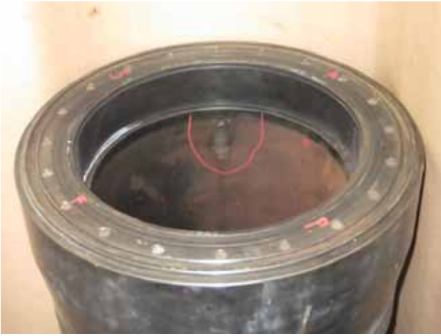
NO.ⓄM216 Poor Conditions specially no uniform touching with Liner and piston ring. 内面当たり不良
