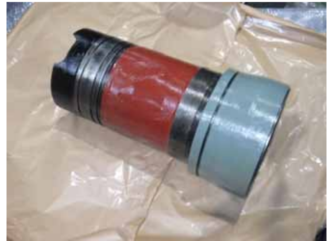
Applied corrosion inhibitor. 防錆剤塗布
