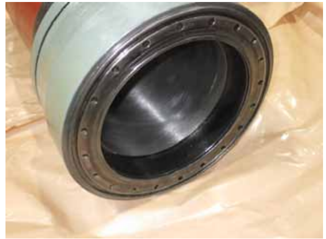
Applied corrosion inhibitor. 防錆剤塗布
