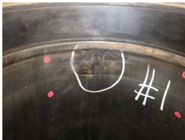
NO.ⓄM210 Poor Conditions specially no uniform touching with Liner and piston ring. 内面当たり不良
