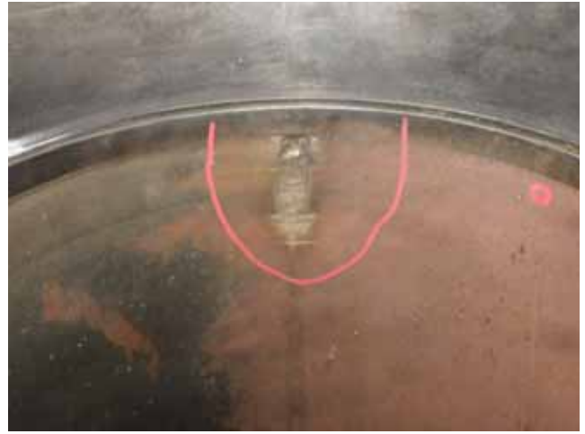
NO.ⓄM216 Poor Conditions specially no uniform touching with Liner and piston ring. 内面当たり不良
