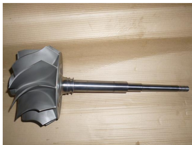
レーザー加工 修正後 [After recondition, Turbine shaft by laser welding.]
